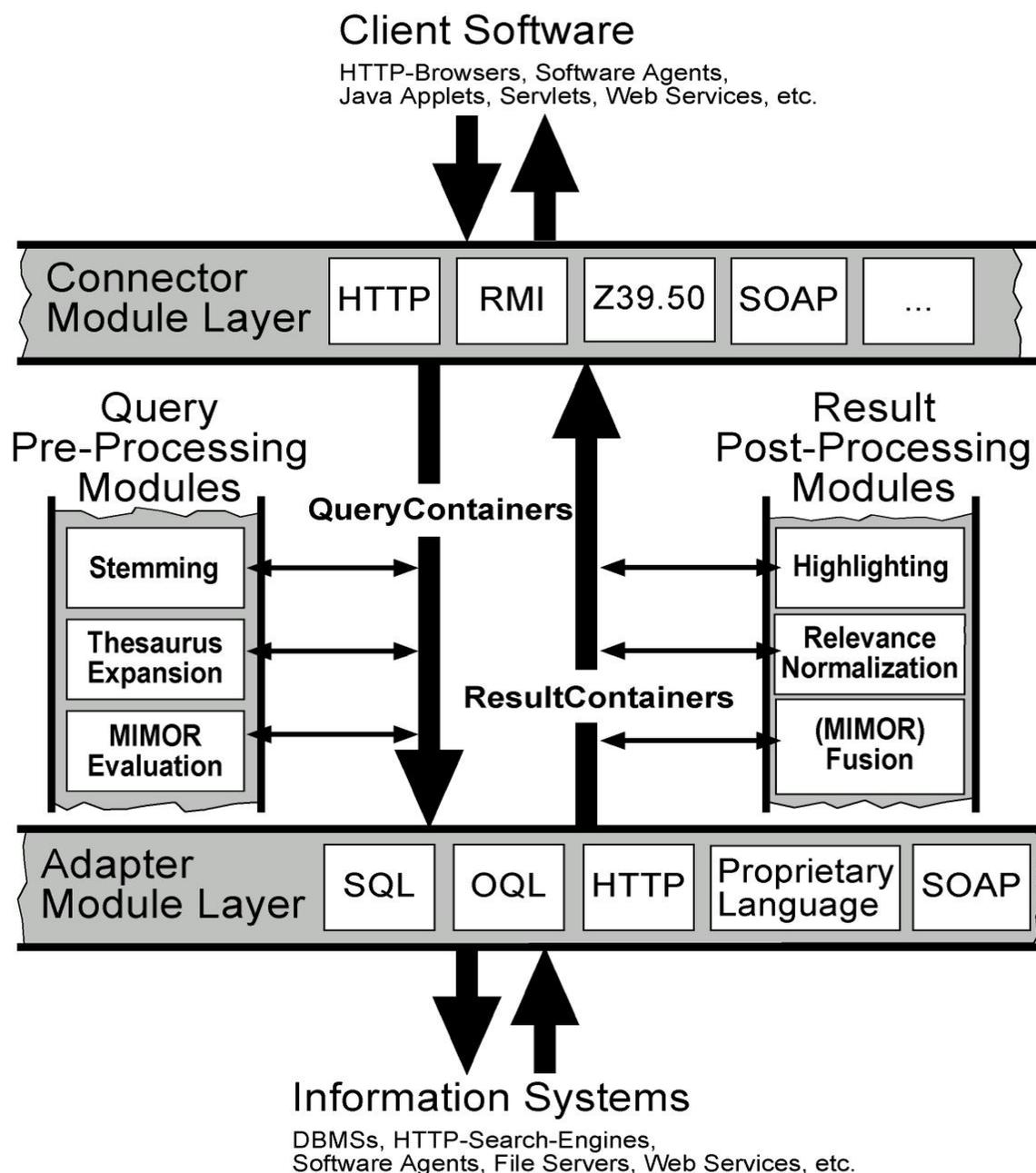
Fig. 2: Three-tier model and inner structure of RECOIN (cf. Kassem 2000:7, Scheufen 2002)
